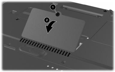
Removing the Memory Expansion Compartment Cover
